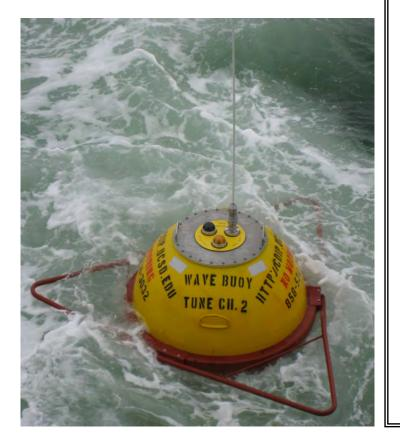
Buoy measures wave height, wave direction, wave period and sea surface temperature.
